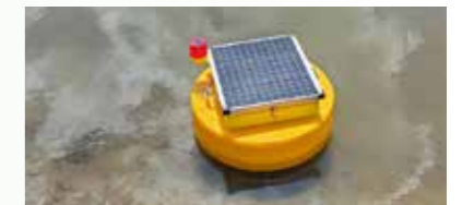
▲ CNMC Luanshya Copper Mines Plc's low-carbon technology innovation (floating automatic water quality monitoring device)
